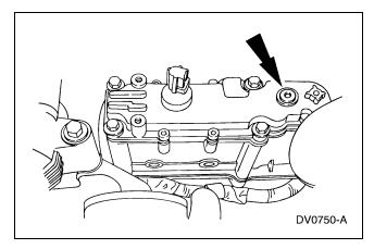
3. Disconnect the engine oil temperature (EOT) sensor electrical connector. Remove the EOT sensor.
