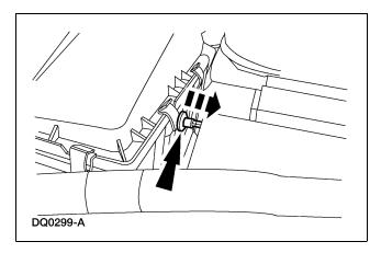
3. Rotate the intake air temperature sensor 1/4 turn counterclockwise and pull outward.
